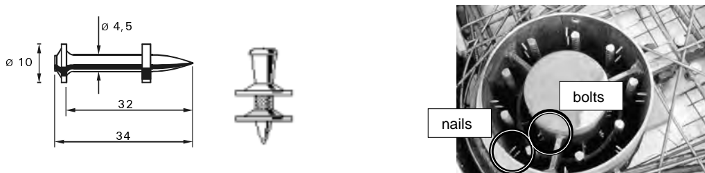
Fig. 7 Shot-fired nails and bolts for shear connection
